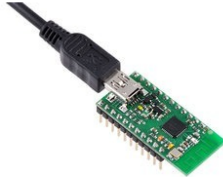
Wixel programmable USB wireless module (fully assembled) with USB cable connected.
