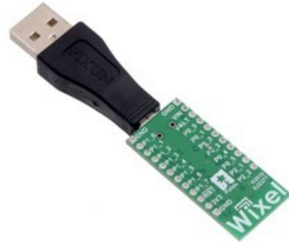
Together, the USB Adapter A to Mini-B and a Pololu Wixel wireless module can make a compact USB dongle.
