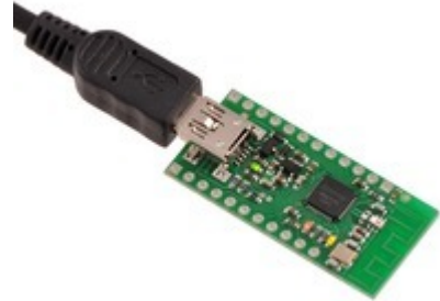
Wixel programmable USB wireless module with USB cabled connected.
