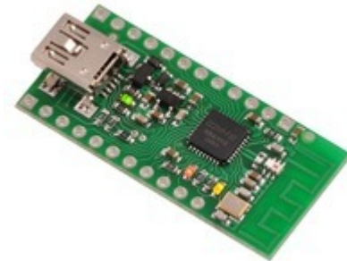
Wixel programmable USB wireless module.
