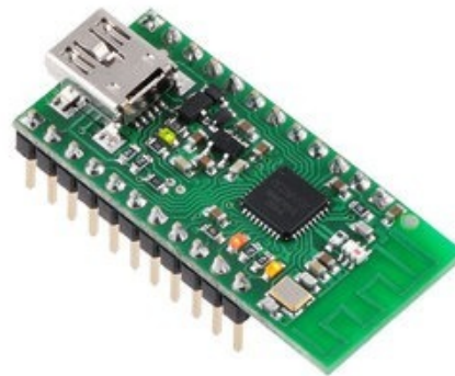
Wixel programmable USB wireless module (fully assembled).
